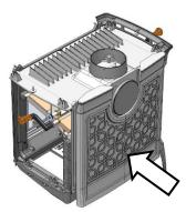
4) Place a bar clamp from the bottom casting to the top casting, as shown below. Apply slight pressure on the clamp and remove the hex barrel nuts from the tie rods on the back of the stove. Pull the tie rods out from the front of the stove.
