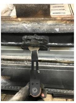
7) Open the ash pan door. Remove the six bolts in the front cast face of the stove. Begin from the right side of the front cast face, pull the cast away from the stove. Be careful to not chip the enamel on the left side of the stove.
