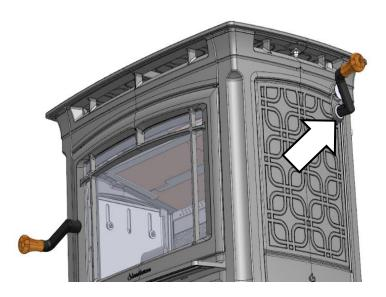
4) Position the bottle jack under the flat face below the ash pan on the right-hand half of the stove. Lift the <u>right side</u> of the stove slightly using a bottle jack, or cribbed wood. The feet must be off the floor at least ½" to remove the side.
