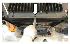
13) Reinstall the six bolts securing the front casting to the primary air plenum. The four longer bolts go on the bottom, the two shorter bolts go on the top.
