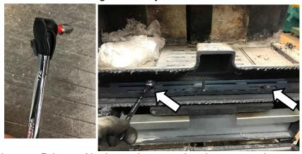
9) Install the new Primary Air shutter by reversing the process in step 8. If hardware is damaged during removal, replacement screws and washers are provided in the kit. Apply anti-seize to the back face of the shutter where it contacts the cast iron. The roller portion of the air shutter should be assembled as seen in the picture below. Note: the hex lock nut must be tightened against the back face of the roller mounting face to ensure the roller does not come loose during use.
