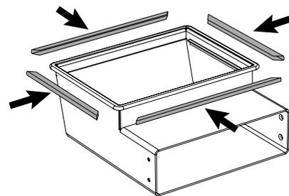
5. Peel white protective paper off of the back of the 1/4" gasket and press it adhesive side down along the top rim of the ash pan box over existing gasket. Be cautious to apply so the outside edges of the 1/4" rope gasket are flush with the outside edges of the ash pan rim. Trim excess to fit with ends touching.
