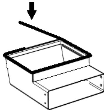
6. Install the ashpan box: Install the ashpan box through the hole in the center of the firebox floor. Position the ashpan box so that the gasketed top rim sits level around the lip of the hole in the cast iron firebox.
