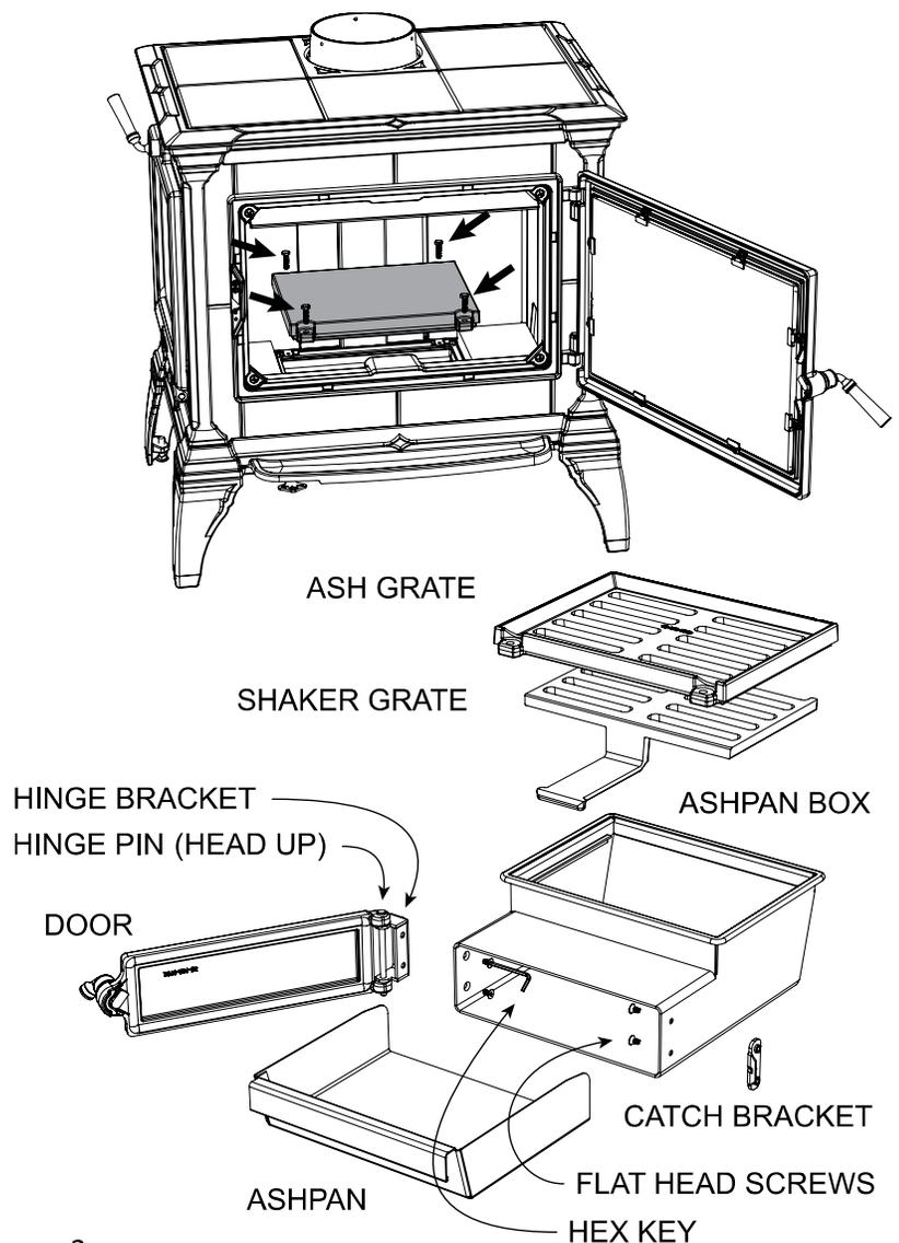
hinge installed on the left side of the ashpan, as the door was shipped.
