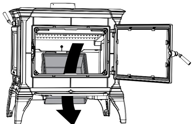
7. Install the shaker grate and ash grate:
